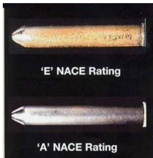
Figure 3 - Shows NACE corrosion examples, A is a passing rating, while E fails.
