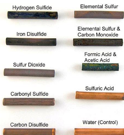
Figure 1 - Examples of Copper Strips Corroded by Various Components
