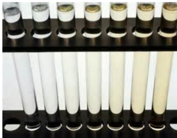
Figure 1 - D1209 Platinum-Cobalt Color Scale Showing Light (5) to Dark (60)
